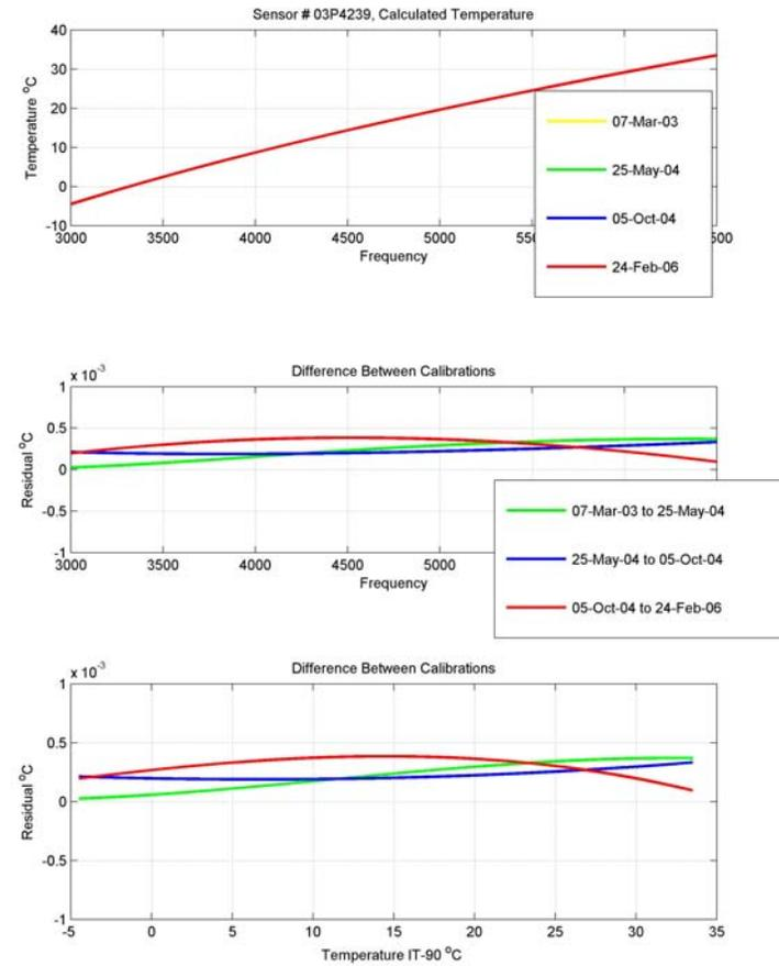
**Figure 7. Lab calibration of (a) primary temperature sensor #4322; and (b) secondary temperature sensor #4239. The red line shows the calibration change for this cruise (from 5 Oct 2004 to 24 Feb 2006).**
